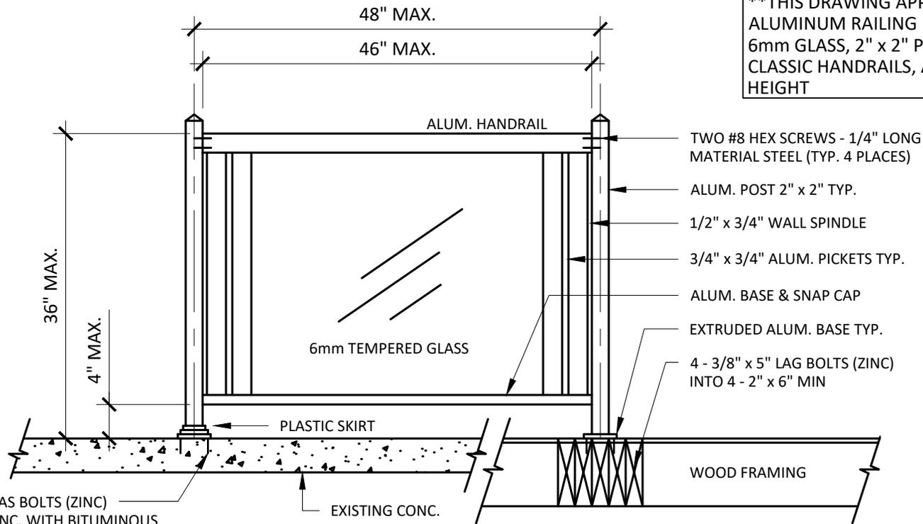
4 - 3/8" x 3 1/2" HAS BOLTS (ZINC) INTO EXISTING CONC. WITH BITUMINOUS MATERIALS IN HOLES, OR 3/8" x 3 3/4" STAINLESS STEEL WEDGE ANCHORS
