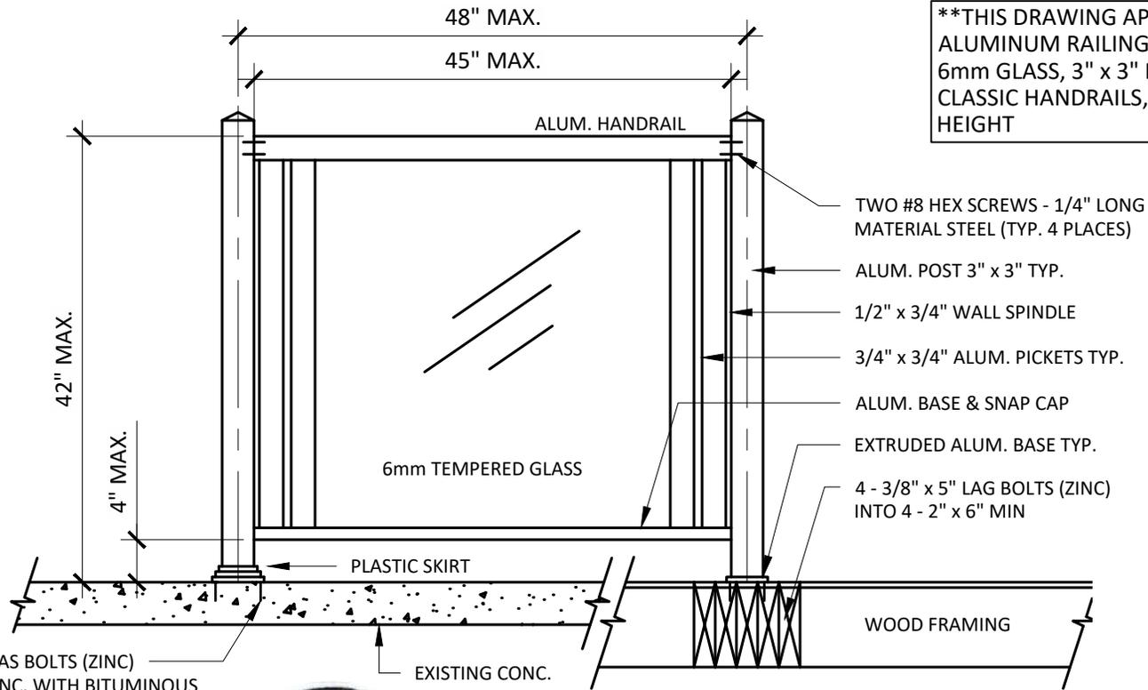
4 - 3/8" x 3 1/2" HAS BOLTS (ZINC) INTO EXISTING CONC. WITH BITUMINOUS MATERIALS IN HOLES, OR 3/8" x 3 3/4" STAINLESS STEEL WEDGE ANCHORS
