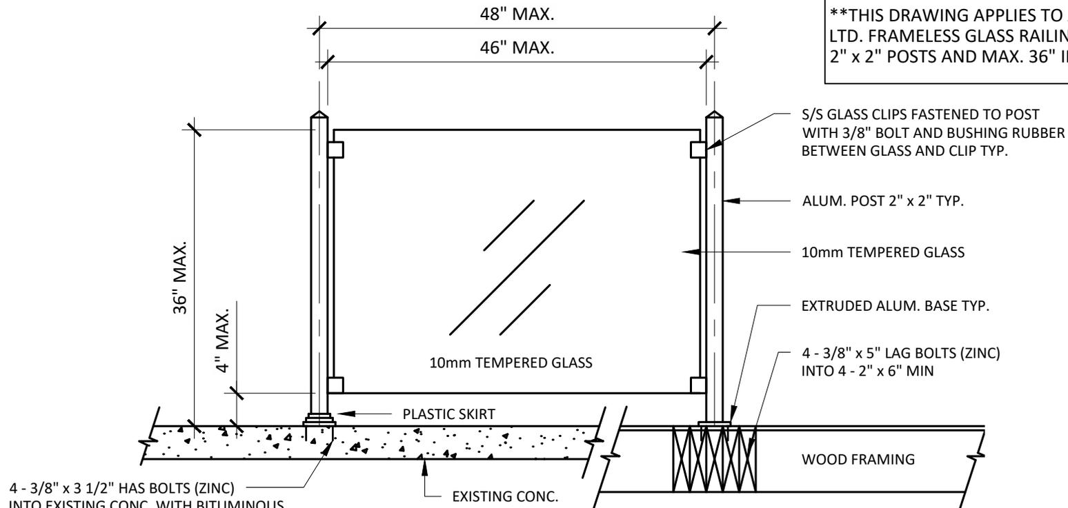
4 - 3/8" x 3 1/2" HAS BOLTS (ZINC) INTO EXISTING CONC. WITH BITUMINOUS MATERIALS IN HOLES, OR 3/8" x 3 3/4" STAINLESS STEEL WEDGE ANCHORS
