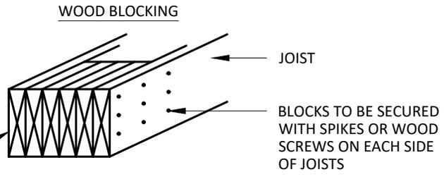
4 - 2" x 8" BETWEEN JOISTS (MIN.)
